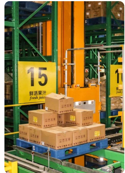
Automatic identification of barcode for stocking
