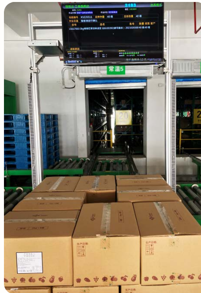
Automatic identification of barcode for storage
