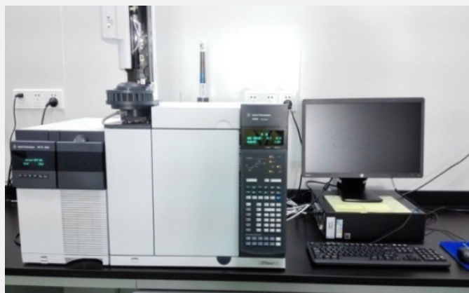
(1) Chromatography chamber – Inspection ingredient for Pesticide residue and auxiliary materials
